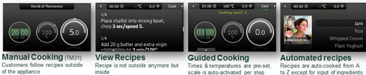
Figure 3: Integration of hardware and software in the TM5 through different cooking modes. 17
